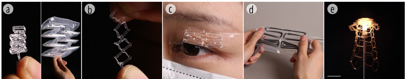
Figure 1: Cross-scale primitive structures and applications of KiriInflate. (a) Comparison of cross-scale primitive KiriInflate; (b) Stretched state of a small-scale inflatable; (c) Eyelid lift assistive device for rehabilitation of ptosis; (d) Multi-mode Interactive game handle; (e) Breathable lamp. (Scale bar: 100 mm.)
