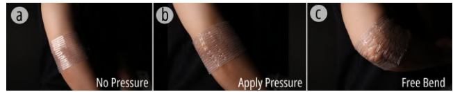
Figure 19: (a-b) Adjustable pressure elbow brace that automatically contracts upon inflation, (c) while allowing for unrestricted bending.
